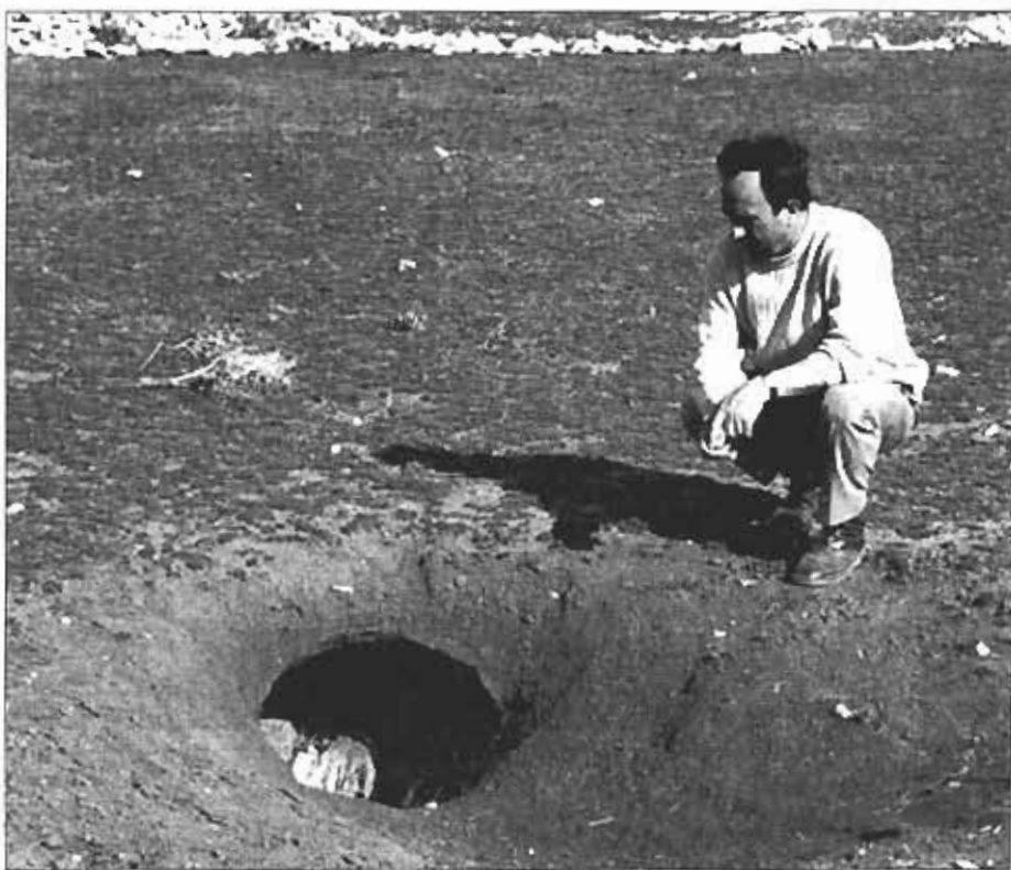
Fig. 10 - Bileca Reservoir. Subsidence created by local water filtration.
